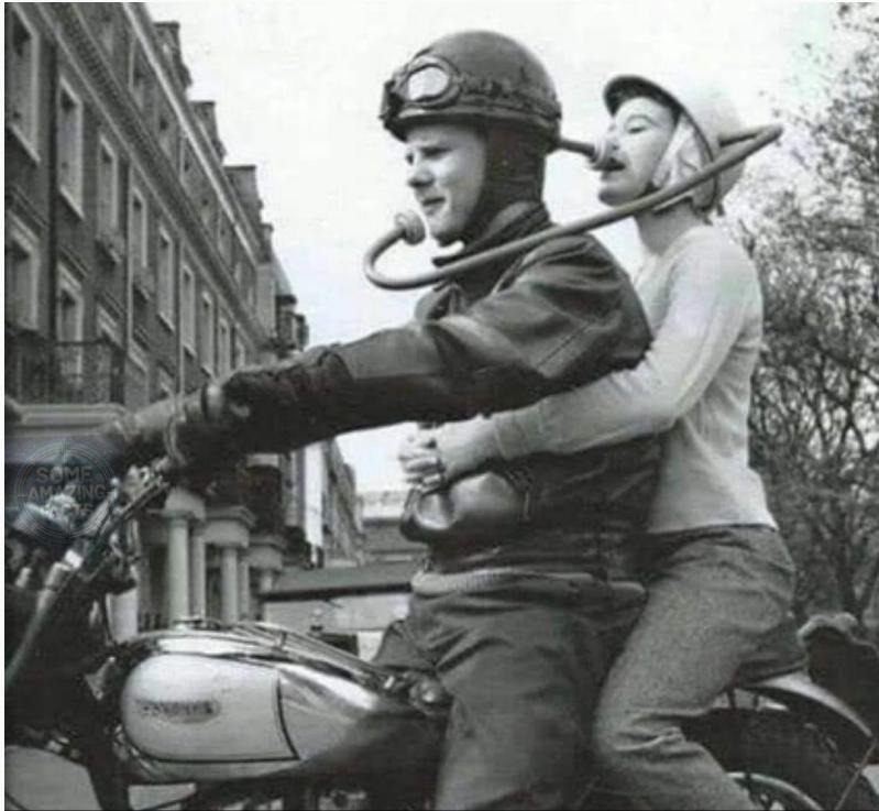
**Early motorcycle riders experimented with helmet-to-helmet speaking tubes in the 1930s–1940s, allowing riders and passengers to communicate acoustically long before electronic intercoms existed.**
