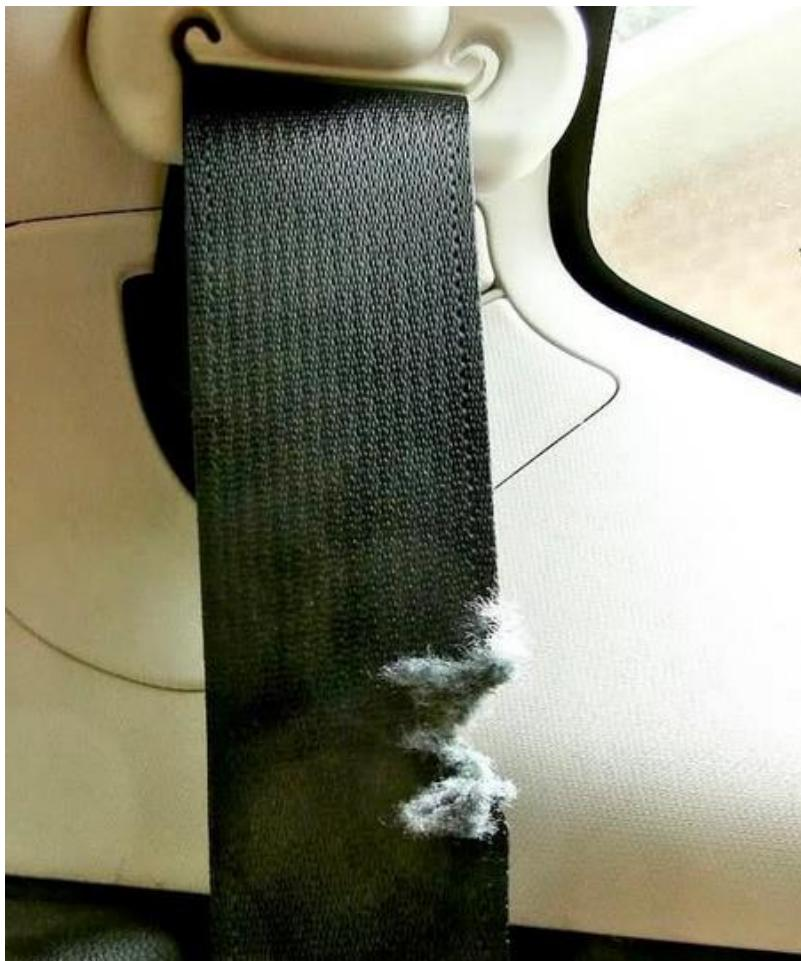
You must immediately stop using the seatbelt and replace it, as fraying compromises its strength and makes it unsafe in a crash.
