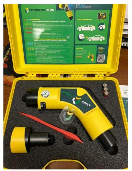
The Town of Peshtigo Fire Department just took delivery of an emergency plug for use on electric vehicles. This device is used to disable an electric vehicle and keep first responders safe when working at an emergency scene involving an EV. This new safety tool will be placed into service and carried on our first
