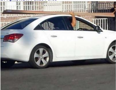
This is NOT an accepted method of restraining a load. â€a#loadfail‬
